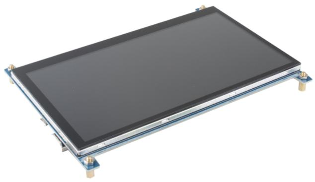
This 7-inch touch screen is compatible with any version of the Raspberry Pi. The kit provides 2 types of HDMI cables, of which HDMI to Micro HDMI cable applies to Raspberry Pi 4 Model B, and the other cable, HDMI to HDMI cable is suitable for Raspberry Pi 3 and the lower versions.
