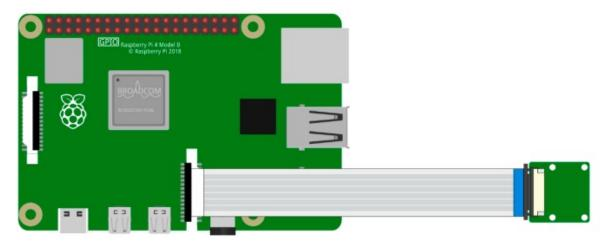
Warning: Do not install the camera with the power on, it may damage your camera.
